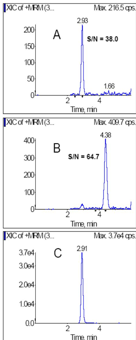
Fig 2. The representative chromatograms of dFdC, dFdU and Gemcitabine-13C, 15N2 at the LLOQ A: dFdC (2ng/mL, 2.93 min); B: dFdU (20 ng/mL, 4.38 min); C: the internal standard (450 ng/mL; 2.91 min) in human plasma
