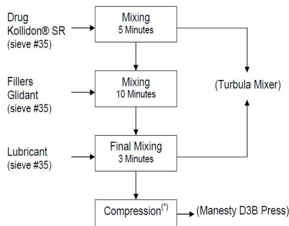
**Figure 1:** Process flow chart for tablets manufactured by direct compression
