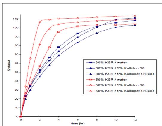
**Figure 7:** Effect of external binder on drug release in water from propranolol 10mg tablets with 30% and 50% Kollidon® SR
