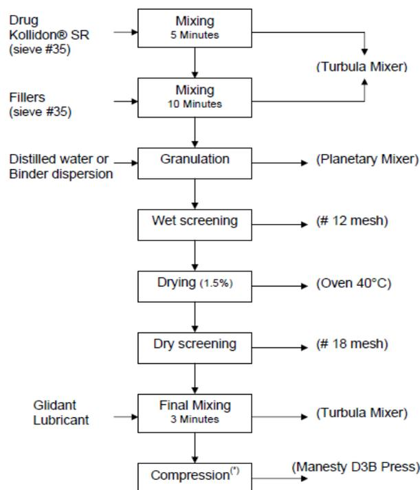
**Figure.2:** Process flow chart for tablets manufactured by wet granulation
