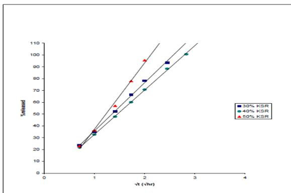
**Figure 6:** Effect of Kollidon® SR on diffusion controlled drug release in water from propranolol 10mg tablets manufactured by wet granulation
