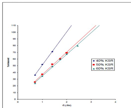
**Figure 10:** Effect of Kollidon® SR on diffusion controlled drug release from propranolol 80mg tablets.
