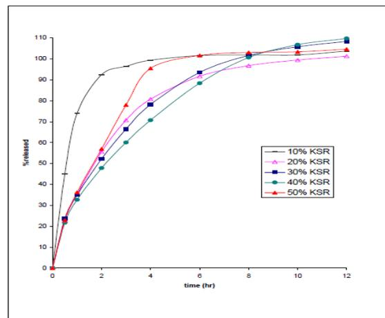
**Figure 5:** Effect of Kollidon® SR on drug release in water from propranolol 10mg tablets manufactured by wet granulation.
