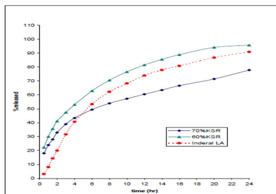
**Figure 15:** Comparison of drug release from propranolol 80 mg tablets with 60 and 70% Kollidon® SR and Inderal® LA.
