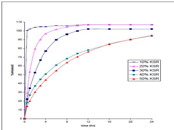
**Figure 3:** Effect of Kollidon® SR on drug release in water from propranolol 10mg tablets manufactured by direct compression.
