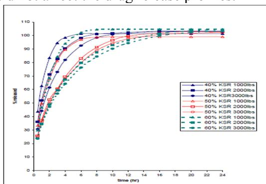
**Figure 9:** Effect of Kollidon® SR and compression force on drug release in water from propranolol 80mg tablets.
