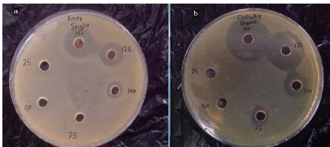
Fig.3. Antibacterial test of a (Fe 2 O 3 ) and b (Ag/Fe 2 O 3 ) against S. dysenteriae in agar medium.
