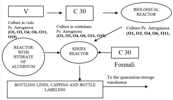
Figure 1 – Scheme of the technological process of manufacturing the vaccine
