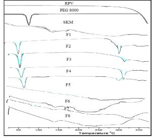
Figure 6: DSC thermograms of rilpivirine, PEG 8000, skimmed milk powder and its solid dispersion systems.
