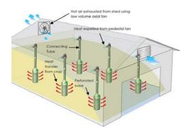
Fig 5: Layout of grain aeration
