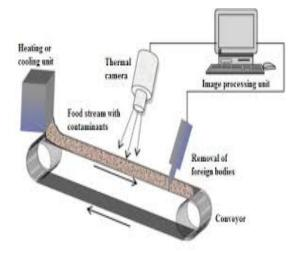
Fig. 16: Temperature in Grains Using Thermal Imaging
