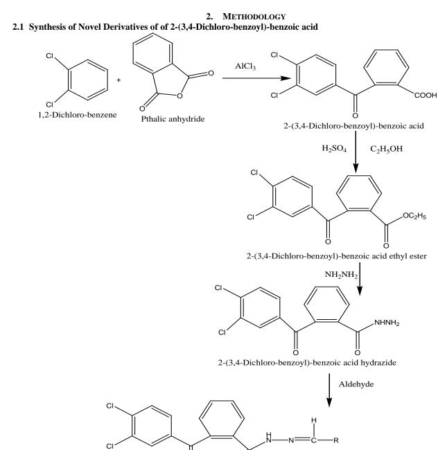
2-(3,4-Dichloro-benzoyl)-benzoic acid (4-methyl-benzylidene)substituted-hydrazide Fig 1: Scheme for Synthesis of 2-(3,4-Dicholoro-benzoyl)-benzoic acid (4-methyl-benzylidene) substituted Hydrazide
