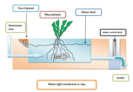
Fig 5. Phytoremediation in constructed wetlands
