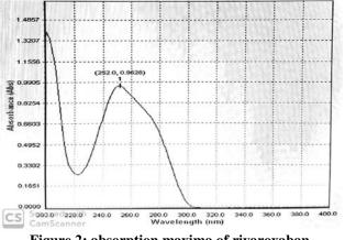
Figure 2: absorption maxima of rivaroxaban.
