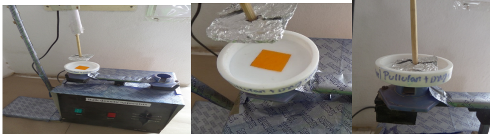
Fig 1: Apparatus for in vitro disintegration time testing of oral films developed by modification of densitometer.
