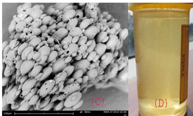
Figure 3. SEM photography C showing the microsphere shape and photography D showing the appearance of microspheres enriched syrup
