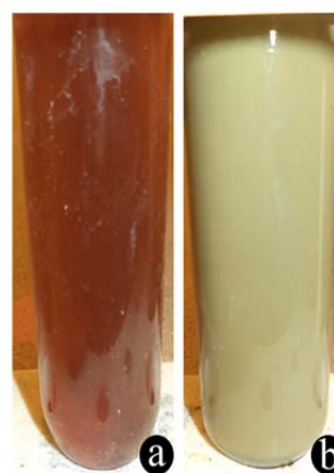
Fig. 2: a) aqueous leaf extract and b) colour change of leaf extract after mixing with \text{AgNO}_3 .
