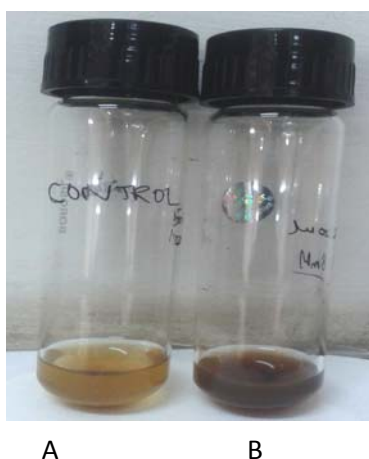
Figure 1: A) Un-inoculated control B) bacterial supernatant containing \text{AgNO}_3
