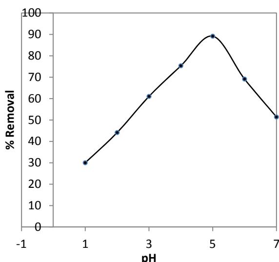
**Figure 1:** Effect of pH on Cu(II) removal by *sea urchin test* for 20mg/L. metal and 0.1 g/30 mL. of adsorbent concentrations.
