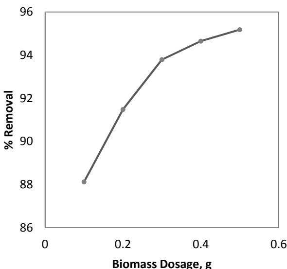
**Figure 4:** Effect of *sea urchin* test dosage on removal of Cd(II) for 20mg/L of metal solution concentration at pH 2 and 80 min of contact time
