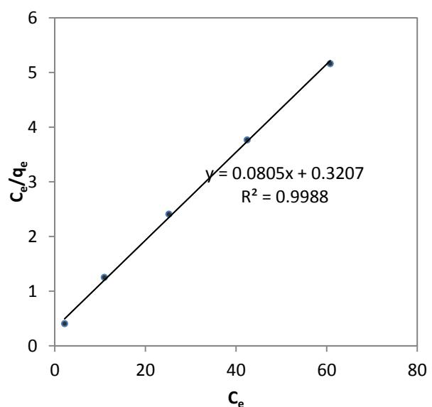
**Figure 5:** Langmuir adsorption isotherm for Cu(II) at 0.1 g/ 30 ml of biomass concentration at pH 5 and contact time of 55 min.
