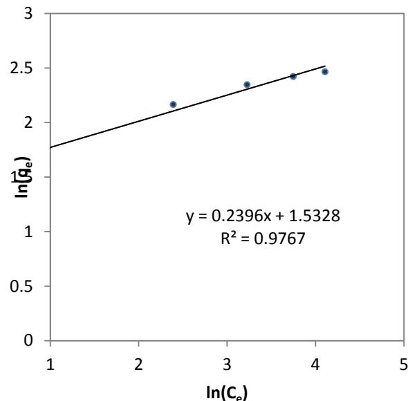
**Figure 6:** Freundlich adsorption isotherm for Cu(II) at 0.1 g/ 30 ml of biomass concentration at pH 5 and contact time of 55 min.
