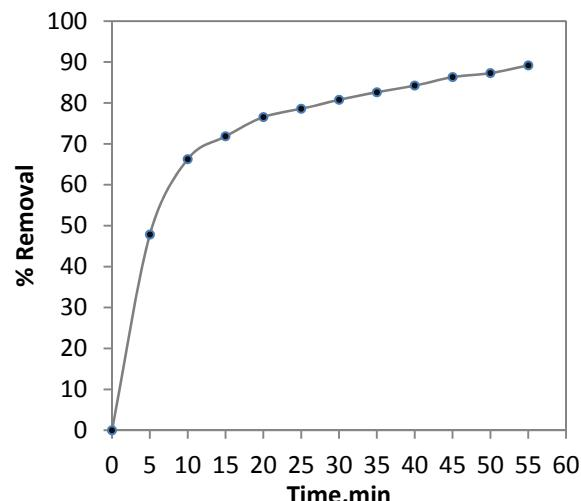
**Figure 2:** Effect of contact time on removal of Cu(II) by *sea urchin test* for 20mg/L of metal concentration and 0.1g/30mL of adsorbent concentration at pH of 5.
