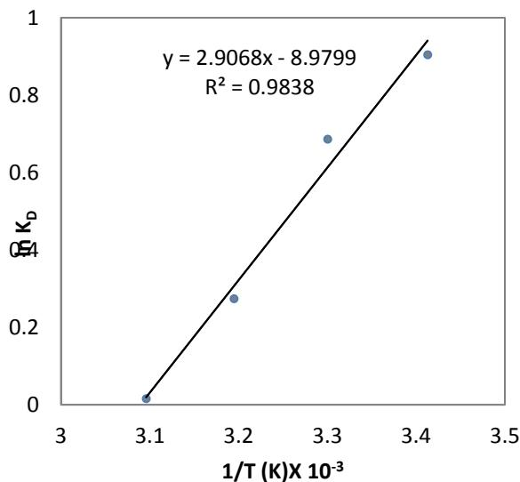
**Figure 8:** Plot of  $\ln(K_D)$  vs.  $1/T$  for the estimation of thermodynamic parameters for biosorption of Cd(II) onto sea urchin test biomass.
