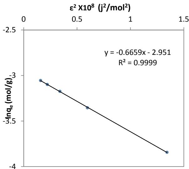
**Figure 7:** Dubinin– Radushkevich isotherm adsorption isotherm for Cu(II) at 0.1 g/ 30 ml of biomass concentration at pH 5 and contact time of 55 min.
