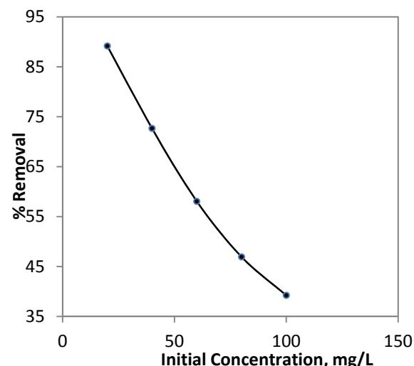
**Figure 3:** Effect of metal ion concentration on removal of Cu(II) by *sea urchin test* at 0.1 g/30mL of adsorbent concentration, pH 5 and contact time 55 min.
