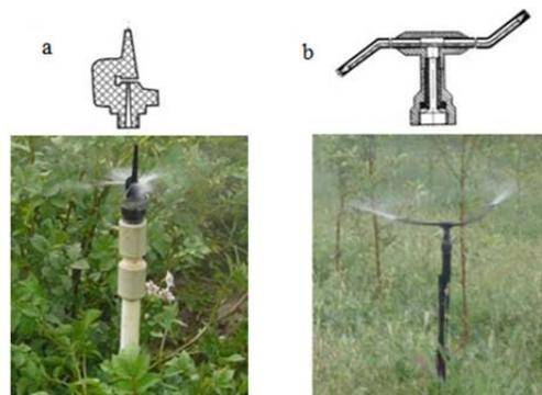
**Figure 3 – Sprinkling nozzles designed by KazSRIWE LLP (a – spray nozzle; b – carousel nozzle)**
