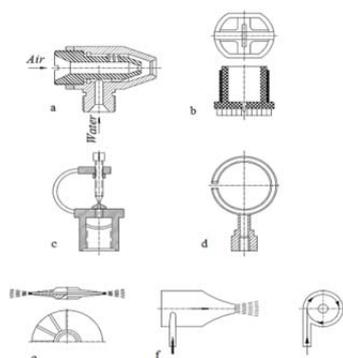
**Figure 1 – Schemes of nozzles of various designs: a – pneumatic spray gun OP-1; b – irrigator PFP-180; c – sprinkler of colliding jets (AFI); d – slit sprinkler; e – rotating disc sprinkler; f – centrifugal spray with vortex chamber**
