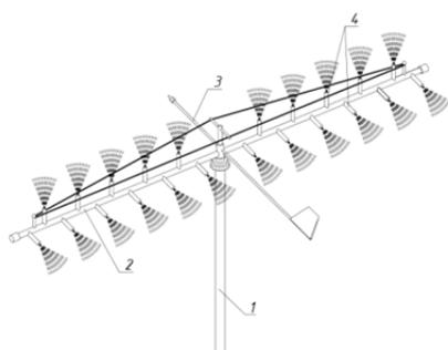
**Figure 2 – Aerosol sprinkling system's rod: 1 – mast; 2 – rotary bar; 3 – weathercock; 4 – dispenser**
