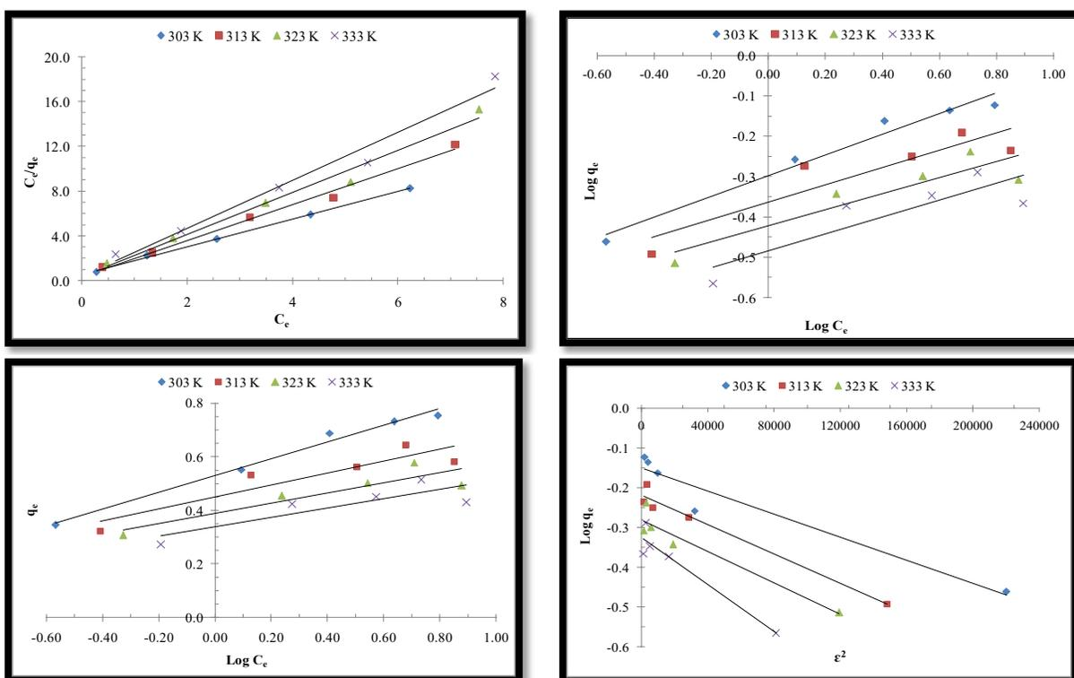
Fig. 2: (a) Langmuir, (b) Freundlich, (c) Temkin and (d) Dubinin-Radushkevich isotherm models for adsorption of fluoride by MACFBL at 303, 313, 323, 333 K.
